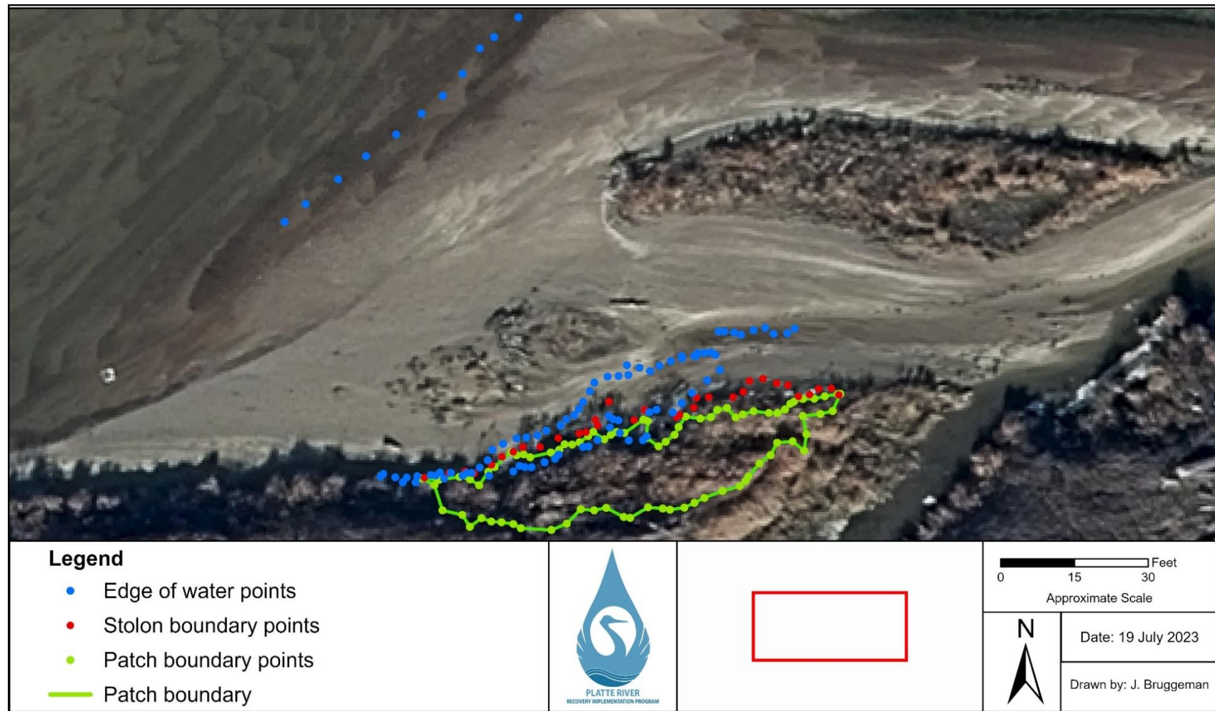
Figure 14. Example of delineated boundaries of a bankline Phragmites patch (green circles and line), stolon reach (red circles), and two edges of water (blue circles) surveyed during May 2023. Circles depict RTK points. Satellite imagery shown is from fall 2022 and does not depict water conditions during the time of the May 2023 survey.
