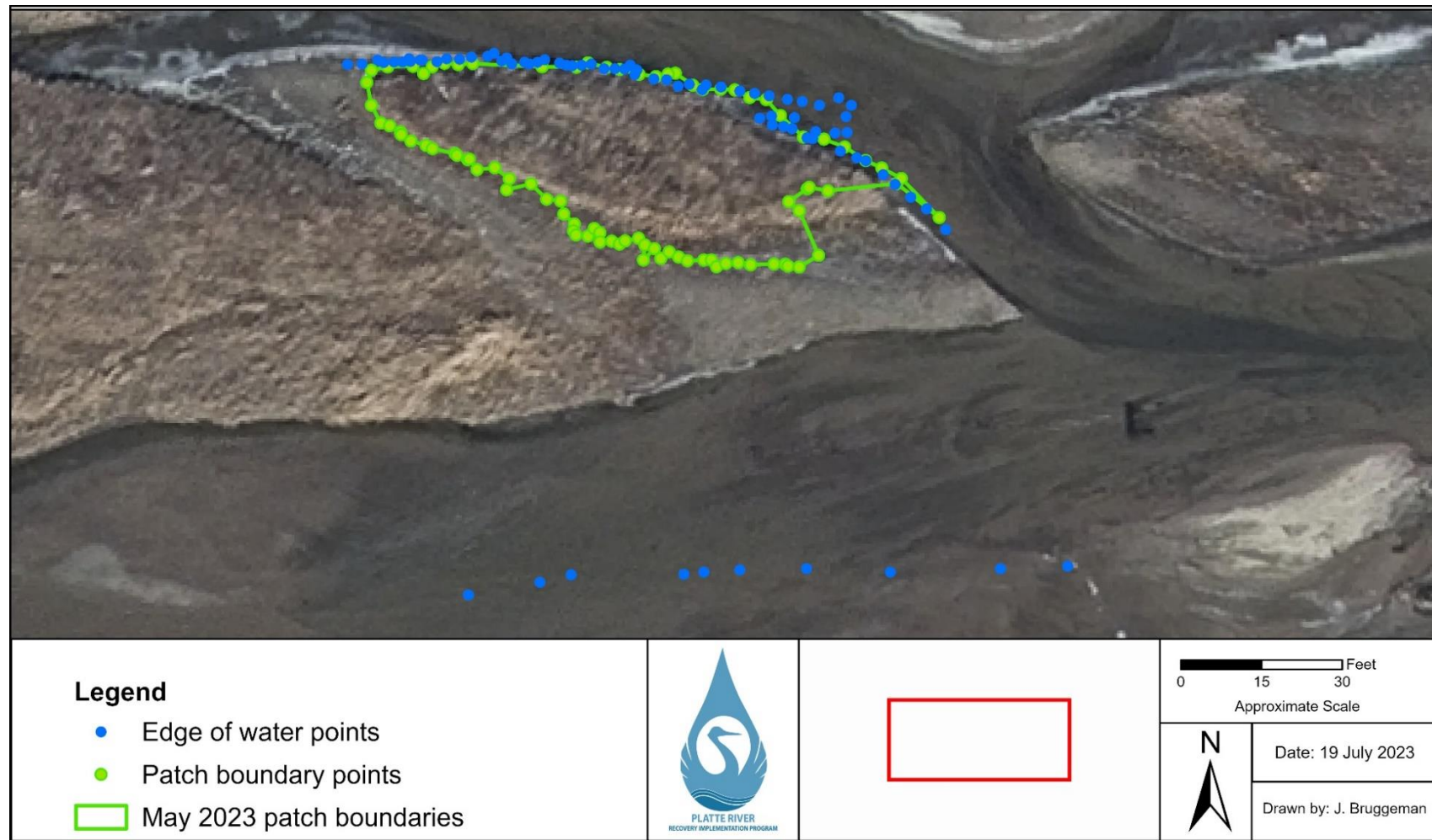
Figure 18. Example of delineated boundaries of an island bankline Phragmites patch (green circles and line) and two edges of water (blue circles) surveyed during May 2023. Circles depict RTK points. Satellite imagery shown is from fall 2022 and does not depict water conditions during the time of the May 2023 survey.
